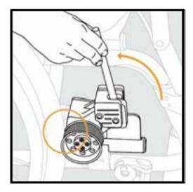
Pull the levers next to both wheels to place the motor wheels in close contact with the wheelchair tires.
