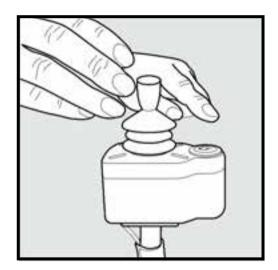
2) After the buzzer rings three times, release the joystick.
