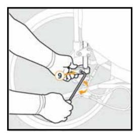
3) Hold the **clamp [9]** loosely on the frame.
