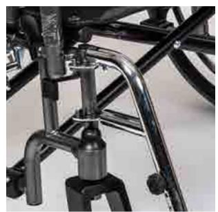
Unscrew the locking pin and adjust the footplates to the desired height before locking the footplate into place.
